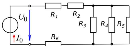
$R_1 = 10 \Omega$ ,  $R_2 = 47 \Omega$ ,  $R_3 = 330 \Omega$ ,  $R_4 = 604 \Omega$ ,  $R_5 = 1000 \Omega$ ,  $R_6 = 11 \Omega$
