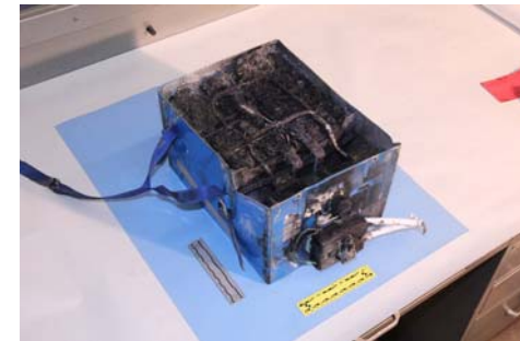
Battery after thermal runaway
